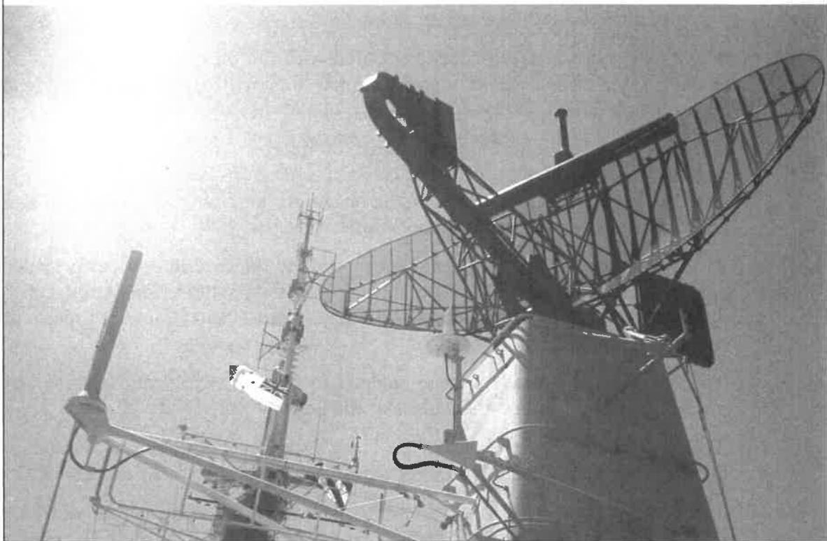
Figure 2 LW08 Radar, installed on HMNZS Canterbury
